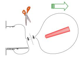
Remove filter cartridge & double tie bag. Cut between ties & discard dirty cartridge. Ensure end cap is positioned as shown. 4
