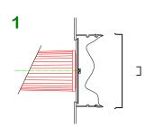
Remove retaining bar & end cover.
